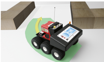
Fig. 1 The SAMS demonstrator driving a right hand bent and the collision-free safety zone of that movement. If there was any obstacle inside the safety zone the AGV would stop.
