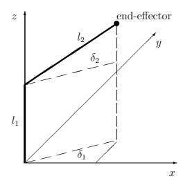
This is a family of robots  $(l_1, l_2)$  are the parameters of the family) with 2 degrees of freedom.
