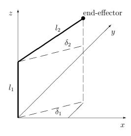
This is a family of robots  $(l_1, l_2)$  are the parameters of the family) with 2 degrees of freedom.
