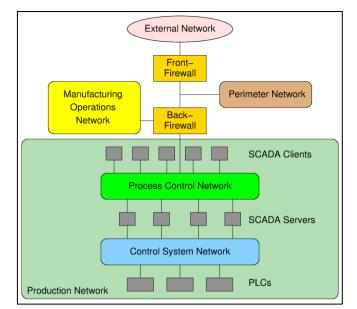
Fig. 1: The network of an industrial process plant.
